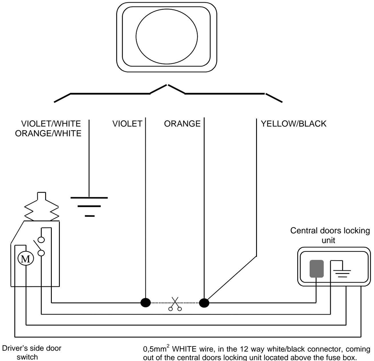
With this diagram, the locking is made with the breaking of the wire, the opening with a ground signal.
