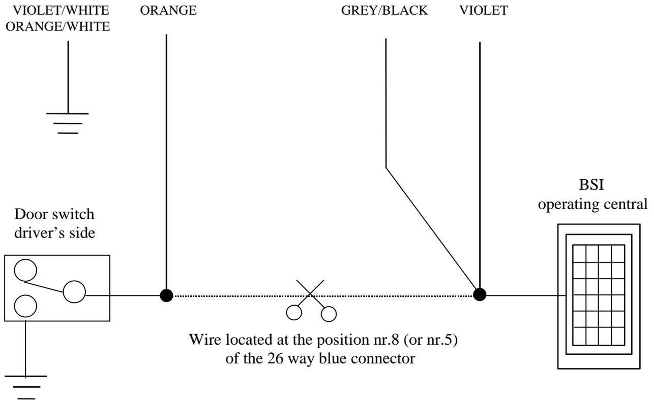
**The BSI operating central is located under the driver's side fuse box.**
