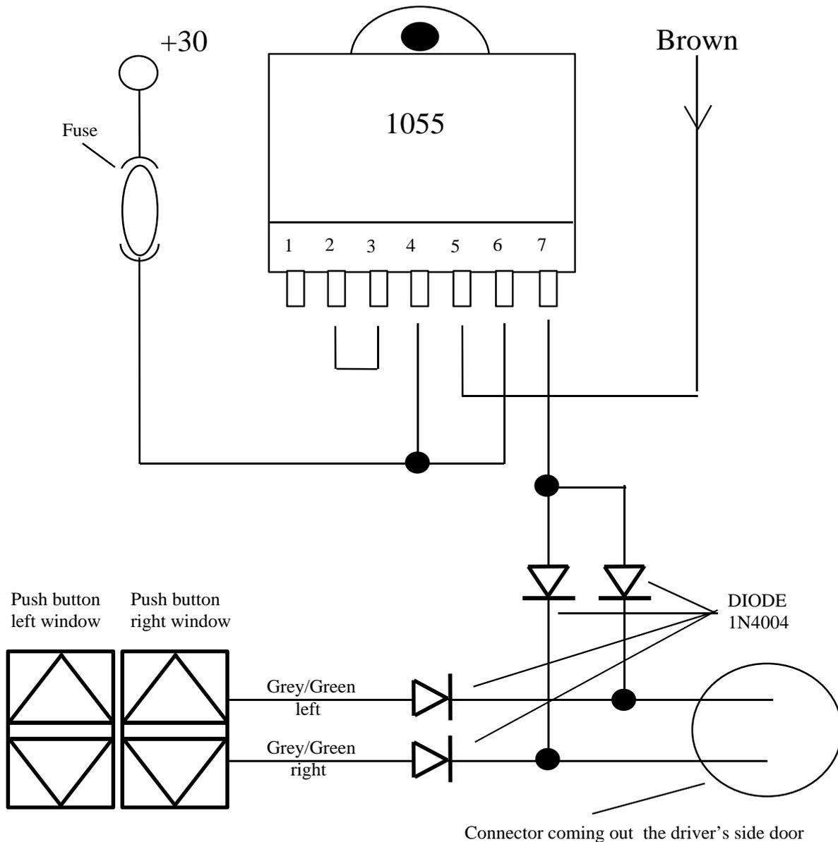
**NOTE:** the windows central unit will reset if it is made a connection between passenger's compartment and door or driving is left for any reason. In order to make a new reprogramming it is enough to operate the window raise for about 5" (when the window is completely closed).
