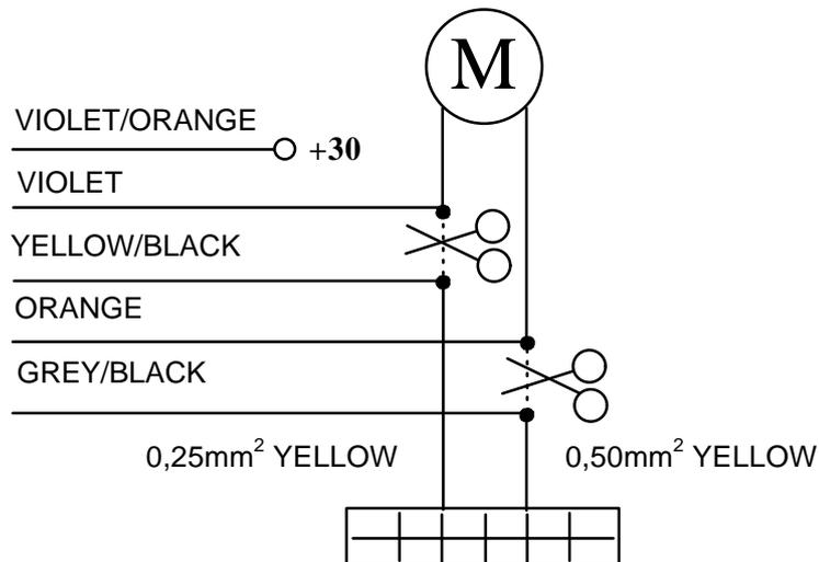
Central locking unit incorporated to the motor inside the driver's side door
