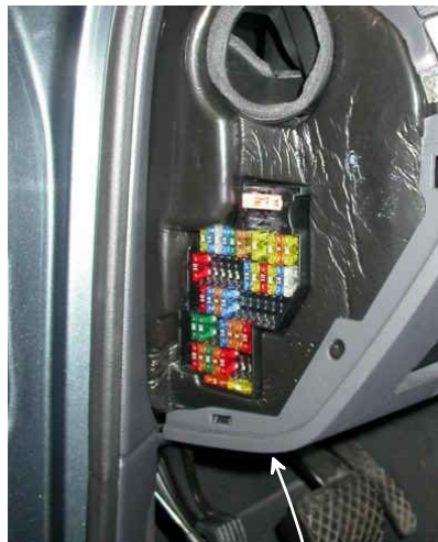
REMOVE PLASTIC COVER TO DISMOUNT RADIO
