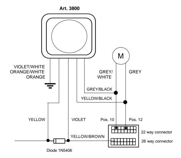
The above connectors are located on the coming out of the central locking unit placed under the glove compartment, in the central tunnel.
