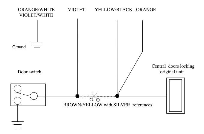
The wire mentioned above is located in the wiring harness coming out of the connector of the driver's side door.
