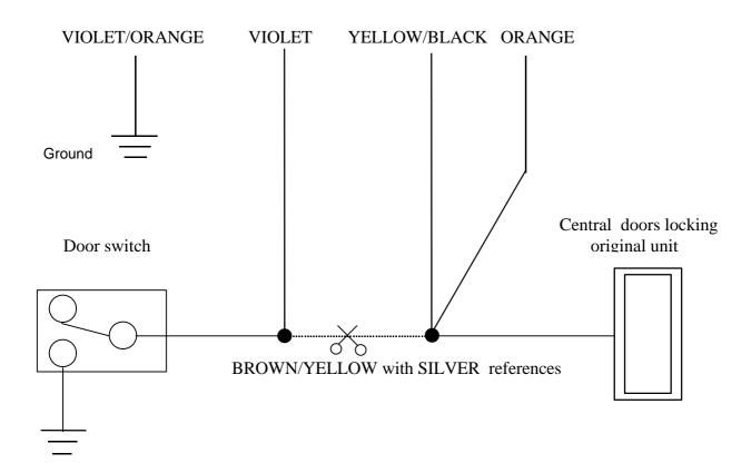
The wire mentioned above is located in the wiring harness coming out of the connector of the driver's side door.
