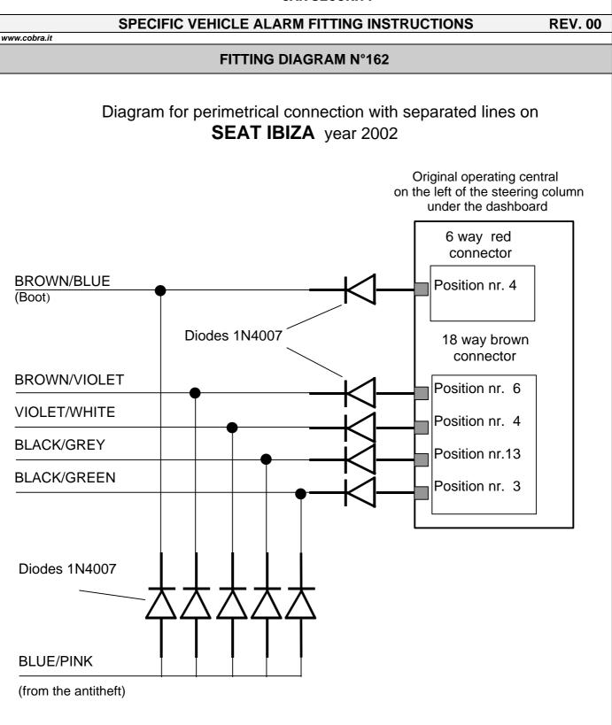
To obtain the perimetrical protection it is necessary to follow this diagram. Each line to the push buttons must be interrupted with diodes in order to avoid false alarms due to negative signals coming out of the operating central of the vehicle.
