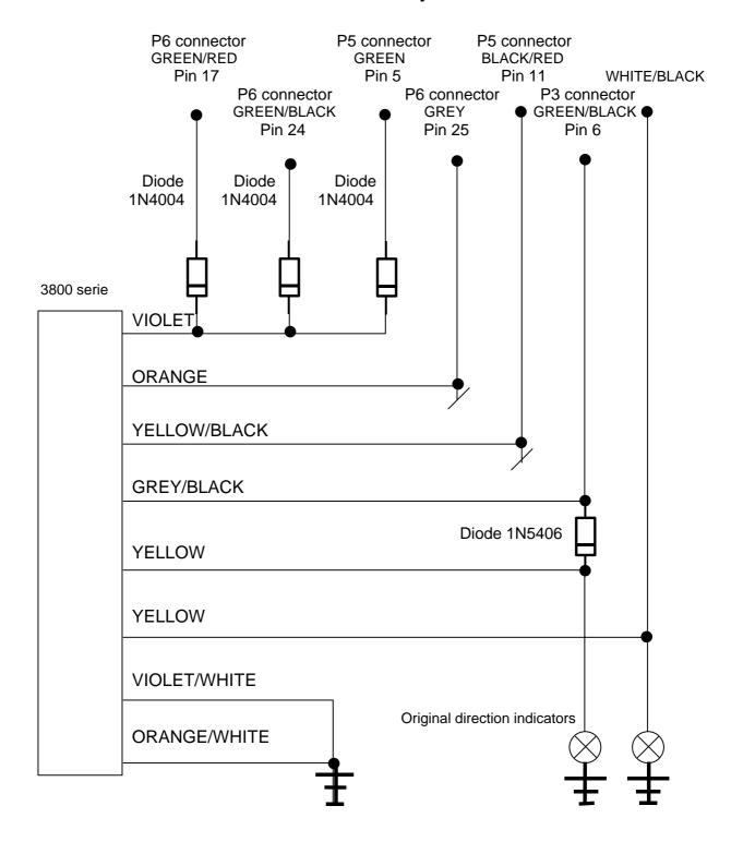
Note: This information is not binding, therefore it must be considered only an example for installation purposes that must be executed as per the instructions given on the product installation manual.
