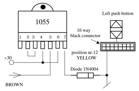
Note: This information is not binding, therefore it must be considered only an example for installation purposes that must be executed as per the instructions given on the product installation manual.
