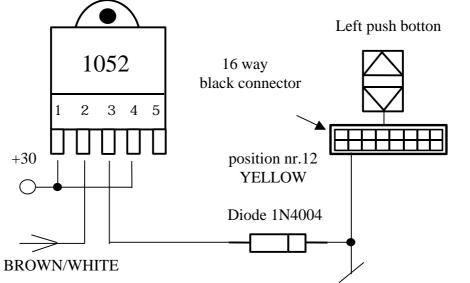
Diagram for windows locking using the BROWN wire of the no autodriven Bridge serie, 3100 and 3800 antith efts.
