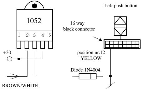
Diagram for windows locking using the BROWN wire of the no autodriven Bridge serie, 3100 and 3800 antith efts.
