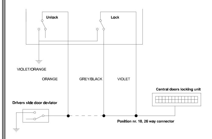
It is necessary to make above connection to lock the doors. The wire mentioned above is located at the position nr.10 in the 26 way blue connector of the central unit of the vehicle, under the driver's side dashboard near the steering column.
