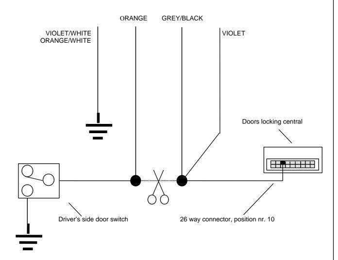
To make the doors locking it is necessary to do the above connection. The 0,35mm<sup>2</sup> wire signaled is located at the position nr.10 in the wiring harness coming out of the 26 way blue connector of the operating central of the vehicle located in the lower part of the driver's side dashboard, near the steering column.
