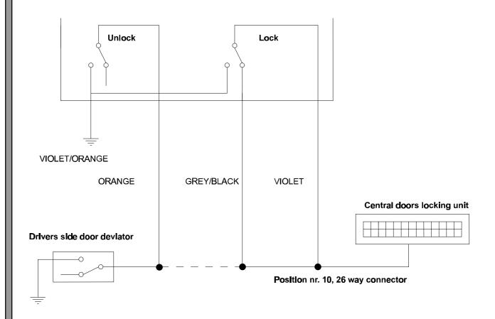
It is necessary to make above connection to lock the doors. The wire mentioned above is located at the position nr.10 in the 26 way blue connector of the central unit of the vehicle, under the driver's side dashboard near the steering column.
