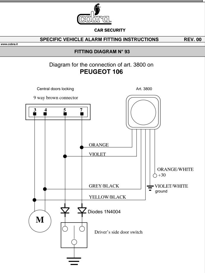
The central unit of the central doors locking is located behind the driver's side air spout. In order to go in it is suggested to take off the annexe pipe.
