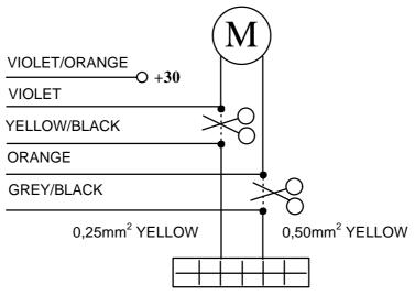
Central locking unit incorporated to the motor inside the driver's side door
