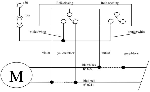
Diagram to connect serial opening/closing doors with radio controls alarms
