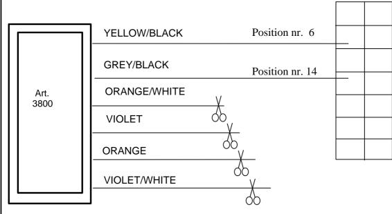
The wires marked with the scissors sign must be cut off near the connector of the antitheft.
