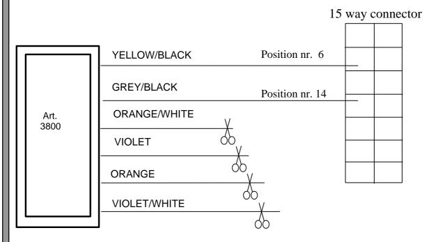
The wires marked with the scissors sign must be cut off near the connector of the antitheft.
